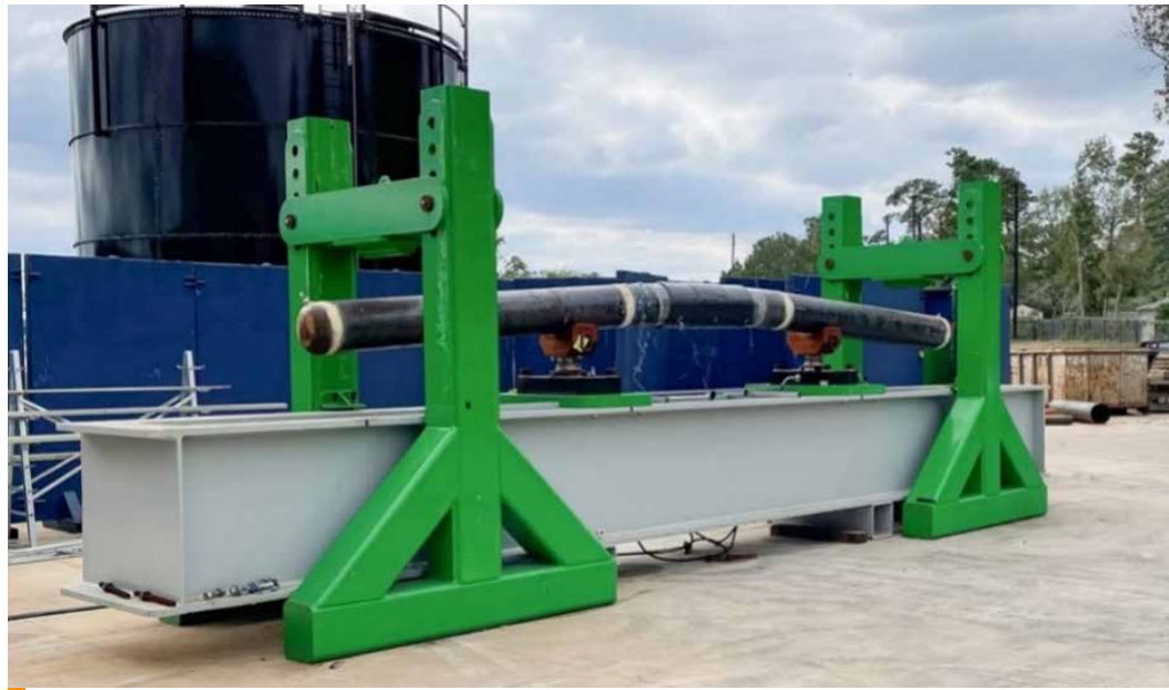
Fig. 4 - 4-point bending frame
