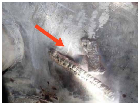
Fig. 2 - External surface of vessel head showing multiple weld repairs and visible deformation (arrow).
