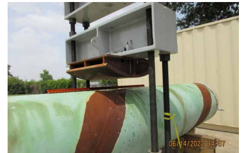
Fig. 1 - Dent installation test rig
