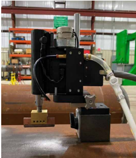
Fig. 6 - Machine used to install EDM notch
