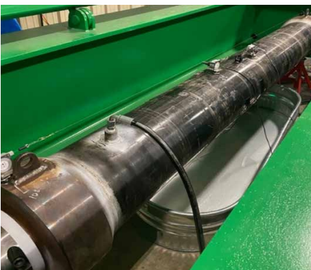
Fig. 3 - Photo and schematic of Acuren's 1-million lbs. tension load frame
