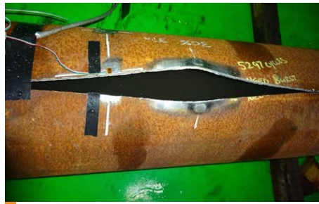
Fig. 8 - Burst test of sample having a crack-like defect
