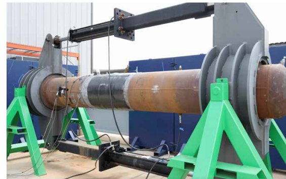
Fig. 5 - High strain bending frame (800,000 ft-lb capacity)
