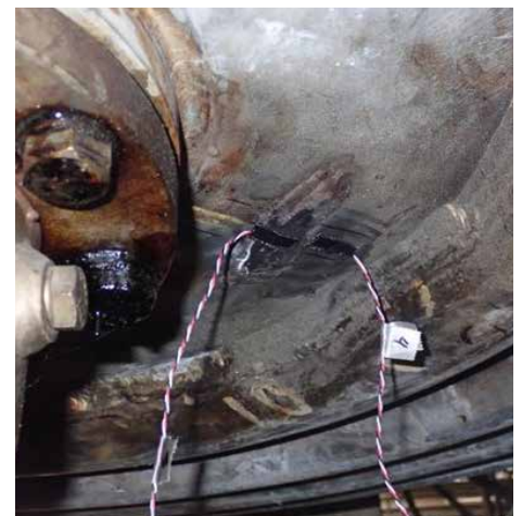
Fig. 3 - Strain gauge placement on vessel bottom head.
