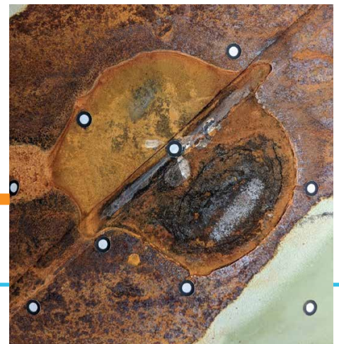
Fig. 2 - Failure of pressure cycled dent
